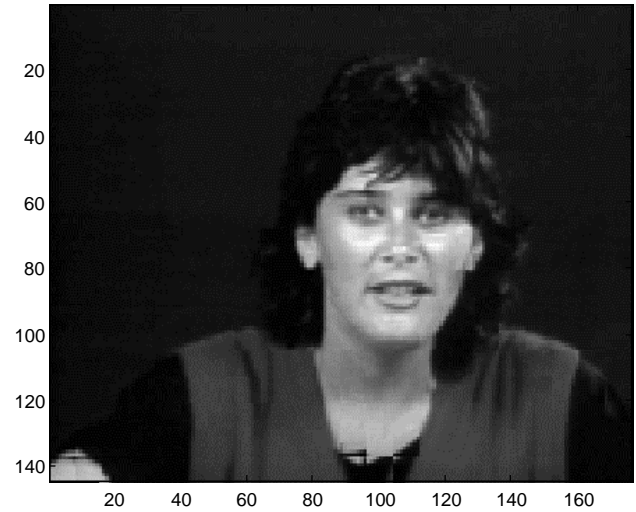
Figure 12. Motion compensated prediction frame resulted from using 8x8 blocks and C=0.25 .
